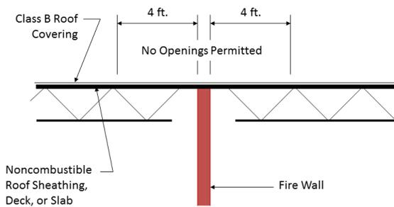
**Figure 12** – Fire wall termination at noncombustible roofs.
