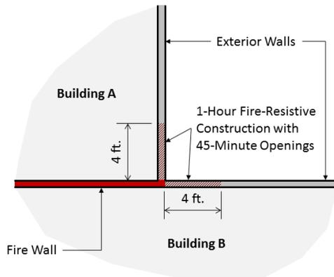
**Figure 1** – Termination of fire wall at exterior walls less than 180° apart using Option 1 simple prescriptive method
