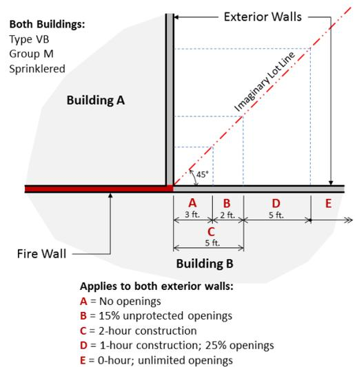
**Figure 2** – Example of terminating fire wall at exterior walls less than 180° apart using Option 2 fire separation distance method.
