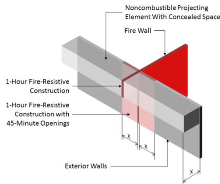
**Figure 7** – Alternate requirement for fire wall through noncombustible projecting element with concealed space.
