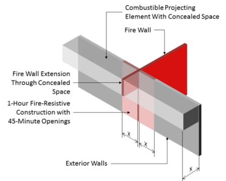
**Figure 8** – Requirement for fire wall through combustible projecting element with concealed space.
