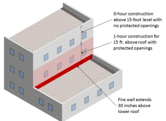
**Figure 10** – Fire wall extension through roof for stepped buildings.
