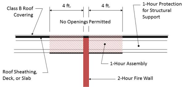
**Figure 11** – 2-hour fire wall termination at underside of roof.
