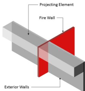
**Figure 4** – Requirement for fire wall through projecting element.
