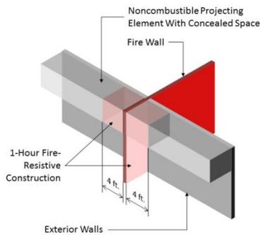
**Figure 6** – Requirement for fire wall through noncombustible projecting element with concealed space.
