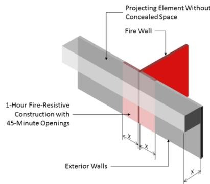
**Figure 5** – Requirement for fire wall through projecting elements without concealed space.
