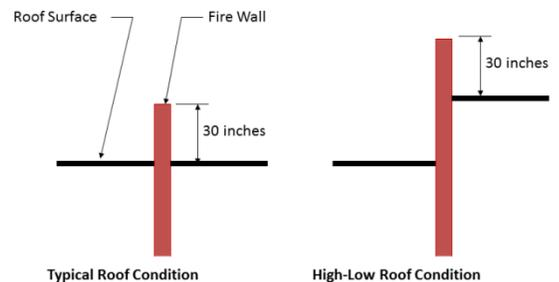
**Figure 9** – Vertical extension of fire wall through roof.
