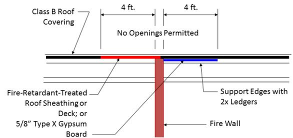
**Figure 13** – Fire wall termination at combustible roofs for Type III, IV, and V construction. Left side shows fire-retardant-treated wood option and right side shows gypsum board application method.
